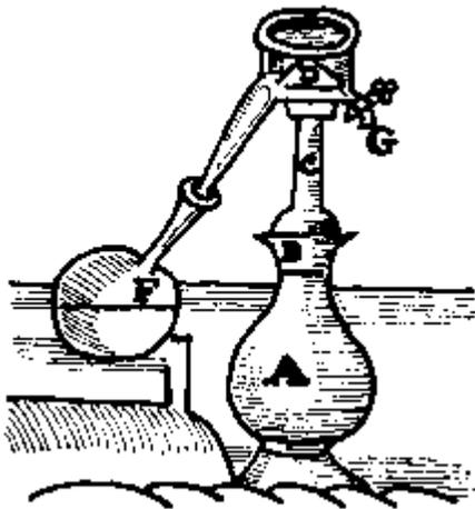
A. Signifies the vessel which must be of copper, in which the matter is contained, and which must be set over a naked fire.
