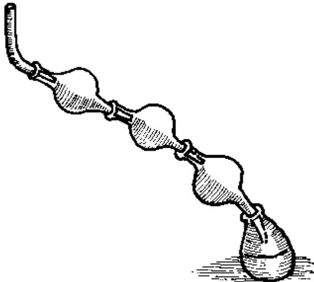
First make your iron vessel as red hot as possibly it can be made (or else you do nothing) having first annexed an earthen well glazed receiver to the bottom of it. Then put half an ounce of quicksilver at a time in at the top (which presently stop with clay) and presently the mercury will come over, part in a sharp liquor and part as crude a mercury as before, which you may put in again until it be all turned to water.
