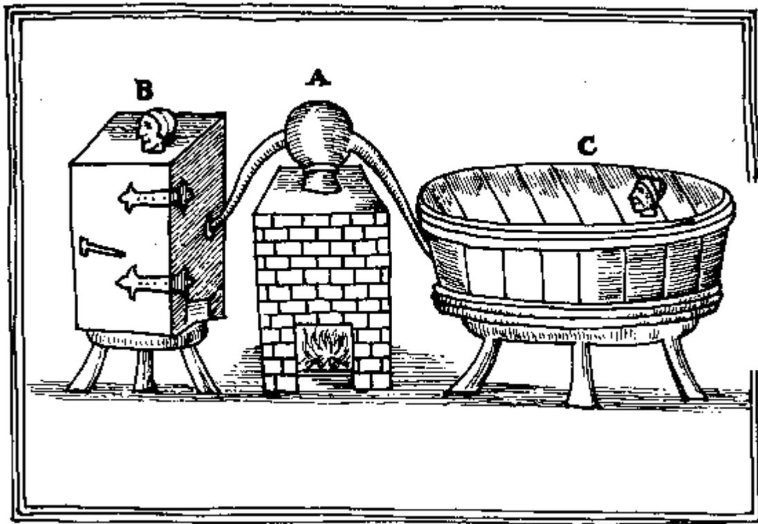
A. Signifies a hot still with two pipes going into two wooden vessels. In this still you may put either herbs, spices, with water or with spirits, and distill them, by which means they that are in the vessels will presently be forced into a sweat by virtue of the subtlety of the vapors. And this indeed is as good and effectual a way for sweating as any can be invented. You may by this means appropriate your ingredients to the nature of the diseases.
