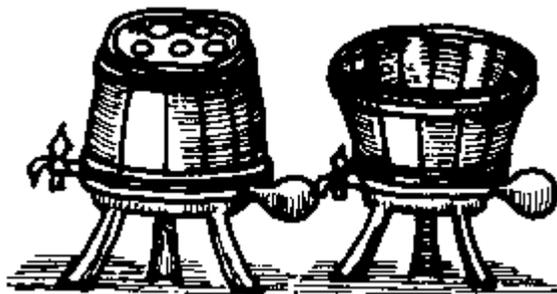
Note that on the right hand these vessels have a copper vessel hanging forth which must be set into a furnace as is above shown. And on the left hand is a cock or tap to let out the water.
