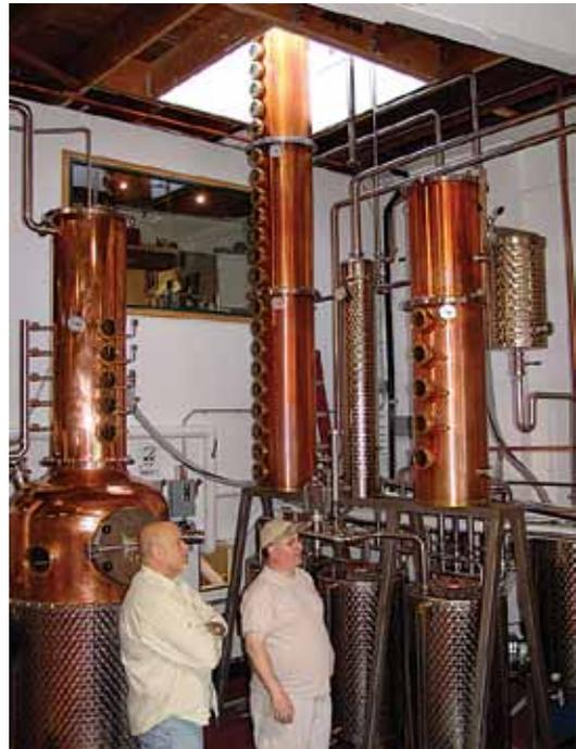
So, when distillation takes place in an artisan still, such as the reflux stills discussed above, the distillate that comes out is divided into three phases called: heads, hearts and, tails. The heads contain the unwanted lower-boiling-point congeners that come out at the beginning of the run, and the tails contain the unwanted higher-boiling-point congeners that come out at the end of the run. And, the hearts are the desired spirit.
